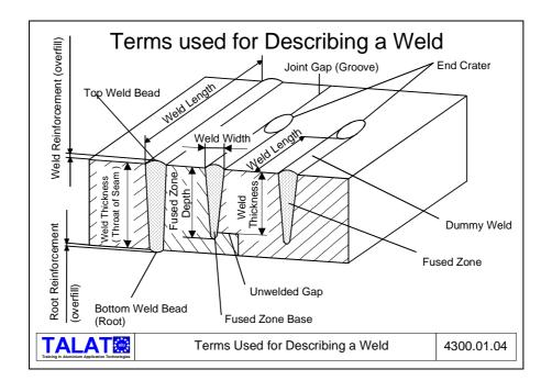
Besides the terms normally used for describing weld joints, one also uses terms like fused zone base and weld thickness or throat of seam, which are specific for electron beam welding. Besides welding, it is also possible to use a reduced beam power for surface treatments like remelting, hardening, engraving etc.
