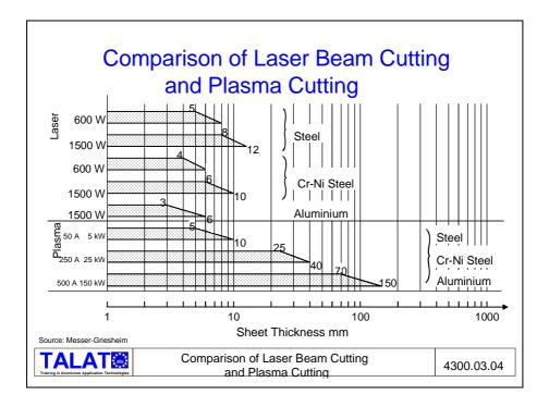
Plasma cutting is ideal for cases in which high quantities are required. The high energy plasma cutting process allows higher cutting speeds, but with lower cut surface qualities and higher distortions than the laser.
