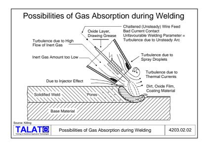
Good degassing of the welding parts and preheating of the work-piece can reduce the gas porosity of welds.
