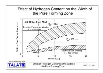
In contrast, the electron beam welding has a very narrow pore formation zone and therefore produces a low weld porosity (**Figure 4203.02.05**). In this case, higher contents of gases in the base material can be tolerated. The influence of welding rate is evident here also. Low welding rates lead to broad pore formation zones and high holding times so that weld porosity increases.
