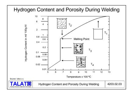
When, during cooling, the melting point is reached, the hydrogen solubility decreases
