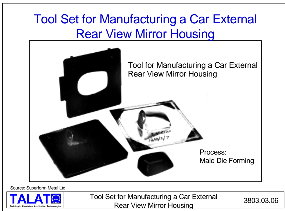
Figure 3803.03.06 shows a tool set, consisting of a punch, punch holder plate and blank holder, for male die forming of an external rear view mirror housing for a car together with an untrimmed and a trimmed component.
