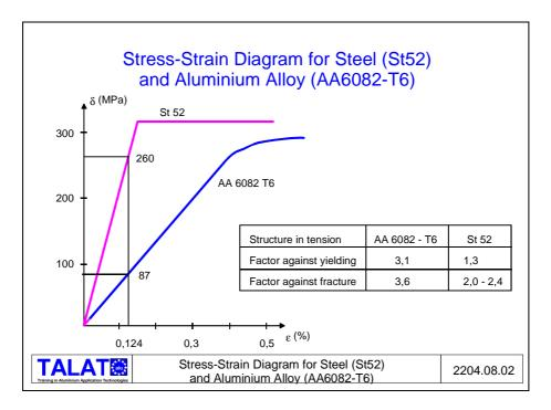
The stress in an aluminium alloy structure designed according to the deflection criteria is very often low. A steel structure will usually be designed according to strength criteria. **Figure 2204.08.02** shows stress strain curves for an aluminium alloy member of 6082-T6-alloy and a steel member of St 52. The example shows different stress in the members for the same strain, caused by the difference in the modulus of elasticity.
