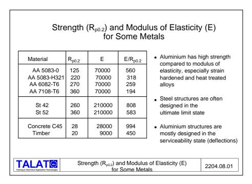
This effect is especially clear when the aluminium alloy is strain-hardened or heattreated. Structural aluminium alloys have roughly twice the strength of steel compared to the modulus of elasticity. Steel designers often use the strength of the material when designing a steel structure, and than check if the deflection is within the requirement.
