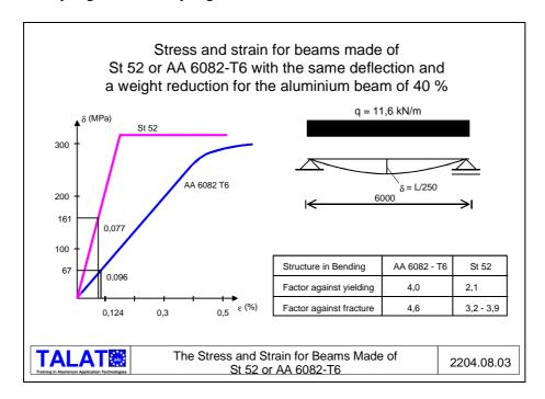
The deflection of members in bending are dependent on the modulus of elasticity (E) and on the moment of inertia (I) together with the load and the span. With the same span and load, it will be the product  $E \cdot I$  which will determine the deflection.
