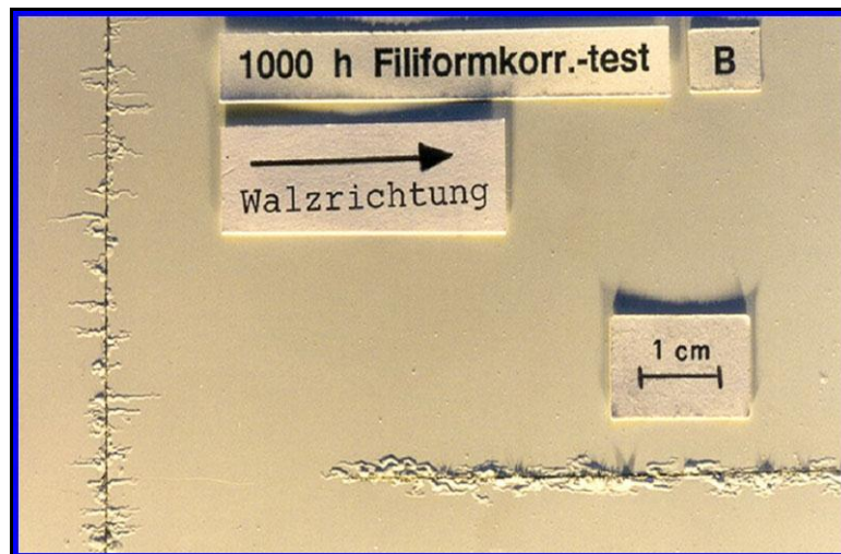
Typical appearance of filiform corrosion: vermicular attack of surface-coated, e.g. painted or anodised aluminium components at the interface metal/coating.
