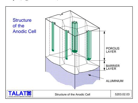
The thickness of the barrier layer depends on the composition of the electrolyte and the operating conditions.
