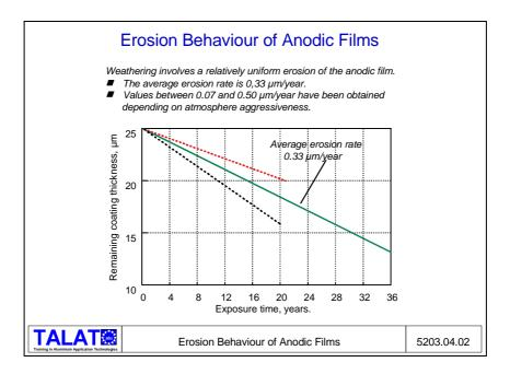
The average erosion rate is  $0.33 \mu m/y ear$ . Values between 0.07 and  $0.50 \mu m/y ear$  have been obtained depending on atmosphere agressivity.
