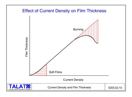
When reflectivity and image clarity are of importance, normally special conditions are used and low current densities in the range of  $1 \text{ A/dm}^2$  tend to improve image clarity.
