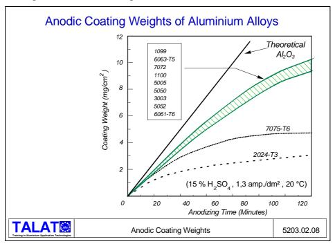
Generally among the aluminium alloys, the series 5xxx y 6xxx produce the best decorative and protective coatings, some 7xxx series alloys also produce clear coatings with good performance. Usually the 2xxx series produce coating colours of inferior quality.
