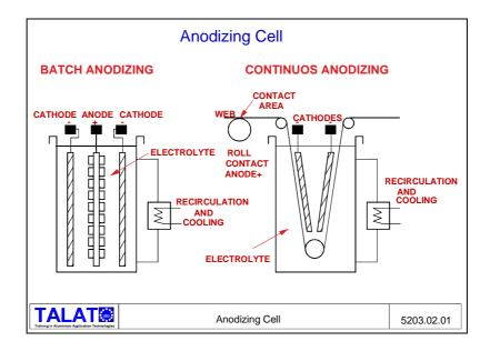
A DC, AC or a combination of both can be used as power supply for anodizing. For standard sulphuric acid anodizing a 24 V rectifier is suitable, however, for chromic acid anodizing or anodizing in organic acid voltages up to 60-70 V are needed. For hard anodizing and for production of barrier-layer films higher voltages are needed.
