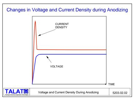
During the initial period of anodizing the aluminium piece is protected by a thin aluminium oxide film that offers little resistance to the current. If anodizing is carried-out at constant voltage a quick rise of current is produced, and later on, a slow drop to a steady
