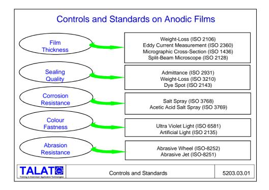
Film thickness in practice is one of the most important control parameters and numerous methods have been suggested. Some film thickness meters are now accurate and dependable (Eddy current measument), but the referee methods in cases of dispute inevitably nivolve destruction of the coating (Micrographic cross-section).
