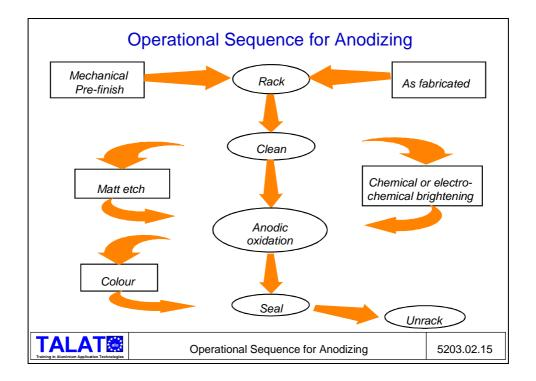
The first step in the anodizing operation is racking. Racking is the operation that provides support and electrical contact for the components being anodized. After racking the material is cleaned in a solution in order to remove: oils, solid particles and even the oxides on surface. Once the material is clean there are three possibilities of treatment: direct anodizing, matt etching or chemical or electrochemical brightening.
