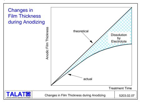
The theoretical value is proportional to the treatment time when anodizing at constant current density acid it depends upon Faraday's Law, which states that the oxide formed is proportional to the electric charge passed (ampere-seconds) through the anode.
