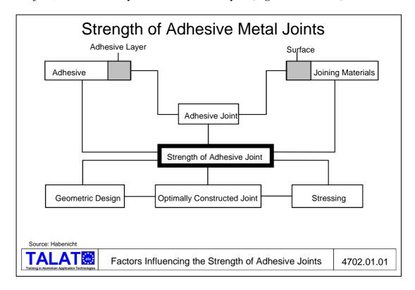
The specific properties of the adhesive joint are a result of the strengths obtained due to the geometrical and material design.
