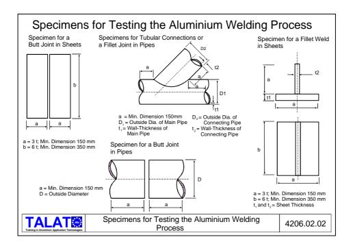
The standard EN 288, part 4, "Requirements and recognition of welding processes for metallic materials", lays down the following specifications for butt and fillet joints:
