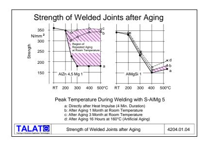
With respect to cracking, the Al-Mg-Si types of alloys are better than the Al-Zn-Mg types of alloys, being less crack sensitive (**Figure 4204.01.04**).
