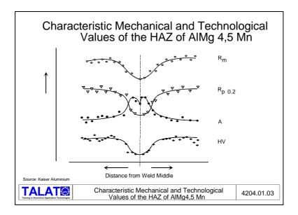
This loss of strength must be considered in designing the welded construction. Calculations should then be based on the reduced allowable stress.
