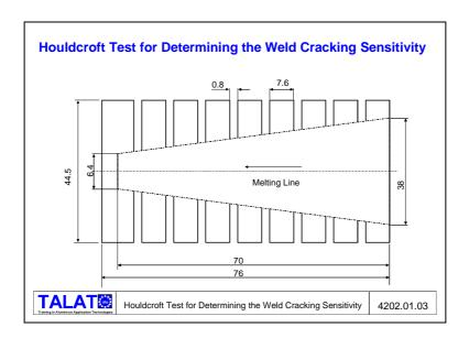
The specimen dimensions, distance between grooves as well as groove width and depth depend on the sheet thickness. At the starting end of the weld in the middle of one side, cracks can form and grow due to the somewhat higher stress existing here. The grooves reduce the stress in steps so that the crack stops growing. The length of the crack formed is an indication of the crack sensitivity of the aluminium alloy tested.
