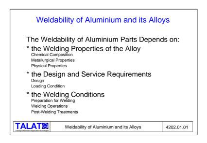
The weldability of aluminium and its alloys depends mainly on the alloy composition, the welding technology and on the notch sensitivity determined by the design (stiffness, residual stress). Some aluminium alloys are susceptible to hot cracking above the solidus line.
