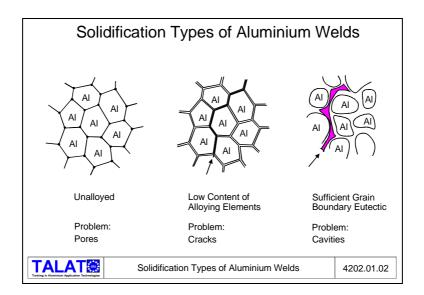
The filler metal must be chosen to ensure a sufficiently large amount of eutectic. Grain boundary movement leads to deformation and material separation. If enough eutectic is available, this can flow in and counteract these defects (**Figure 4202.01.02**).
