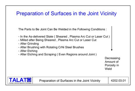
Mechanical or chemical methods are essential for high quality, reproducible welds (**Figure 4202.03.01**).
