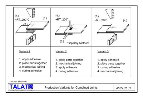
In the so-called "capillary" method, a mechanical joint is first prepared and then an adhesive of low viscosity is brought into the joint crevice. In this variation - which is characterised by a clear separation of the parts to be joint - the adhesive serves generally as a sealant and/or as an inhibitor for corrosion.
