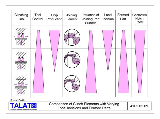
This means that reducing the incision part amounts to an increased effort in aligning punch and die (Figure 4102.02.09).
