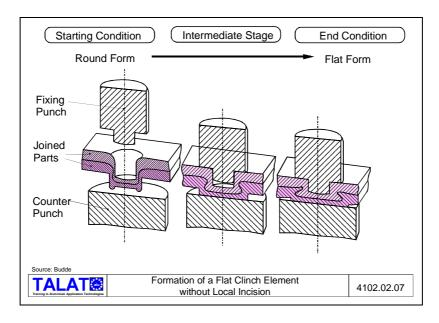
Similar to clinching with local incision, it is possible, in a two-step or multi-step process, to produce a clinch element without local incision (Figure 4102.02.08).
