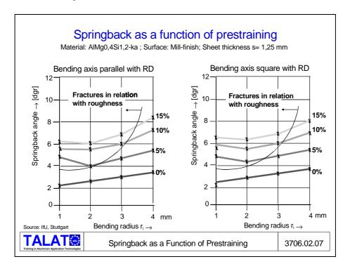
It is clearly evident here that the springback also depends on the position of the bending axis with respect to the rolling direction. For the sheets in mill finish condition shown here, the springback angle is higher when the bending axis is at  $90^{\circ}$  to the rolling direction than when it is parallel to the rolling direction.
