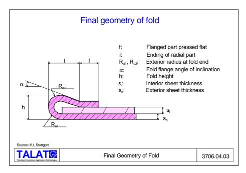
**Figure 3706.04.03** illustrates that the outside radii of the fold edge  $(R_{a1}, R_{a2})$  of a bead fold can be varied. These radii depend on the inside bending radius  $r_i$  used for the 90° bending as well as on the geometry or angle  $\alpha$  of the final folding punch.
