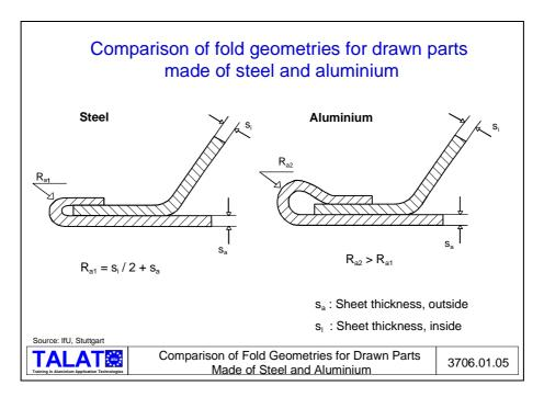
In summary, steel and aluminium have different forming behaviours which make it necessary to use different designs for folding tools.
