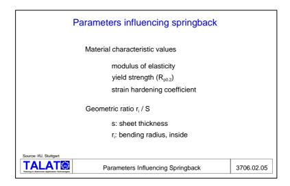
By proper choice of the geometrical ratio the smallest bending factor  $r_i/s$  can be determined for which failure is not encountered and the springback is minimum.
