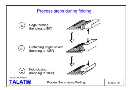
Body parts are mostly folded in presses, in which the forming operation is carried out over the whole rim of the part in two or three steps, unlike the partial round folding of cans. The principle steps of the operation are shown in **Figure 3706.01.04.** In the first step, the edges of the outer radii are bent to 90°. In the second step, the edge is bent another 45° (bending to 135°, prefolding). In the third step, the fold is press closed (bending to 180°, finished fold).
