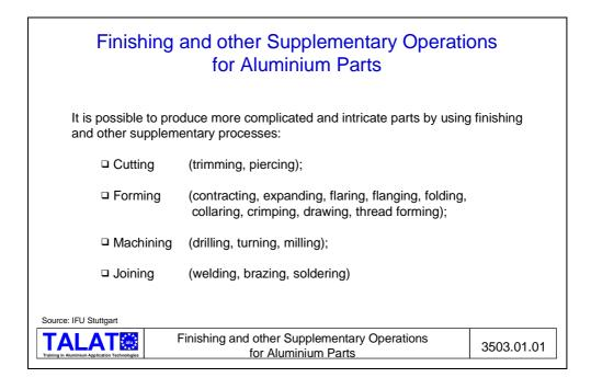
**Figure 3503.01.01** and **Figure 3503.01.02** describe choices and criteria of supplementary working or finishing processes of aluminium impacts.
