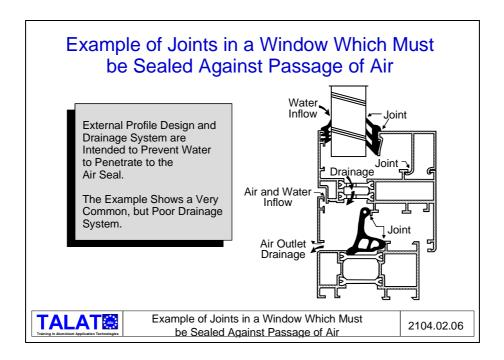
Generally speaking, the drainage system will consist of a collection channel on the sill and lower window profile, which must have a minimum dimension. Likewise the drainage holes which will conduct the water away, should have a minimum dimension (**Figure 2104.02.07**).
