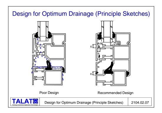
The dimensions are determined by the size of a water drop which is approximately 4.5 mm in both the horizontal and vertical planes. A drainage channel or hole must therefore be larger than 4.5 mm such that the surface tension in the drop does not cause it to adhere to the sides of the channel or holes, and thus prevent satisfactory flow before it has built up a water level within the channel which then may push the water towards the air seal.
