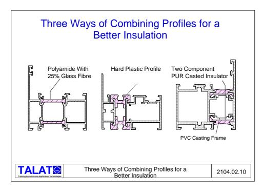
Mainly an extruded polyamide strip, reinforced with 25% glass fibre is introduced into a track in the profiles and clamped. This substance allows thermo-setting <u>after</u> surface treatment up to 200 °C approximately, which means that the profiles can be assembled before surface treatment. This reduces the risk of damage to the surfaces in the event of assembly taking place after treatment.
