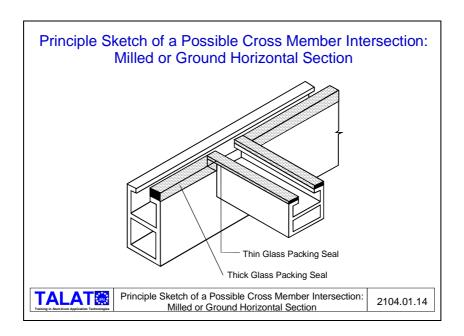
A requirement of both solutions is that the connection between the aluminium sections must be watertight. This is achieved using a ready-shaped rubber sealant covering the sides and the base of the horizontal section, and which is compressed as the horizontal section is fastened to the vertical section at the intersection. Grouting used as a sealant in these areas usually has a short service life, and will require frequent maintenance (**Figure 2104.01.15**).
