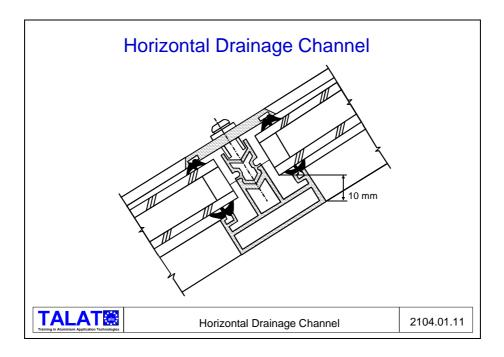
In the case of facades, the aim is to drain out any penetrated water through holes in the horizontal cross member of each piece of glass. With a roof, however, the water will try to penetrate into the sections.
