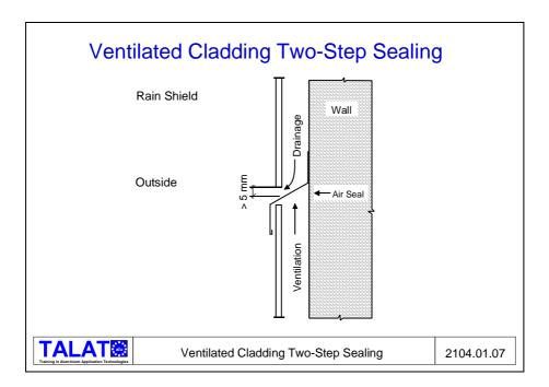
If the wind seal is moistened by the rain, the drop in pressure will occur over the film of water which has formed over the wind seal, and as it does not have the properties to withstand pressure, it will puncture at the weakest point of the wind seal, with guaranteed leaking to the inside (**Figure 2104.01.08**). If the rain is not allowed to come into contact with the wind seal, this kind of leakage never takes place.
