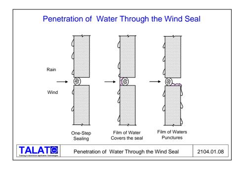
Sections in glass roofs must, therefore, always be designed such that penetrated water must never come into contact with the wind seal (Figure 2104.01.09).
