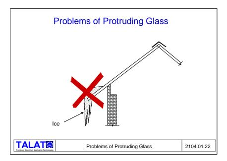
The combination of glass roofs and different, well-insulated roof surfaces may cause the formation of ice. If the insulated roof is above the glass roof, and the glass is directed downwards towards a final outlet drain, then the roof will work well. Snow will remain of the insulated part and melt on the glass roof.
