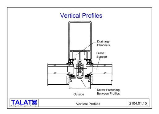
A horizontal drainage channel should also be deeper than 5 mm to prevent water coming into contact with the inner glass packing. A certain amount of flexing of the horizontal
