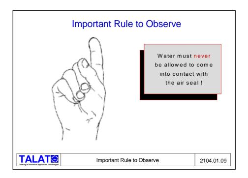
This principle is applied in vertical facades and most types of windows with good results. Glass roofs should not be an exception. We know from experience and tests that seals exposed to the outside never remain absolutely watertight for a long period, and so
