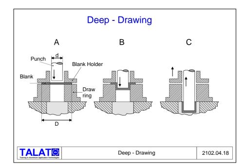
Figure 2102.04.18 illustrates how this drawing process works:
