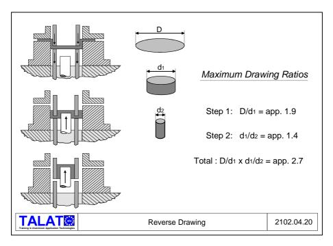
The advantage of reverse drawing is that two drawing operations are completed in one and the same machine operation. The table shows that we can expect a maximum total deep-drawing ratio of  $1.9 \times 1.4 = 2.7$  (if we assume the material is in a soft state). The cup can be drawn using a mechanical or a hydraulic press. More complex operations like reverse drawing demand precision adjustment of the drawing parameters, so a hydraulic press is preferable.
