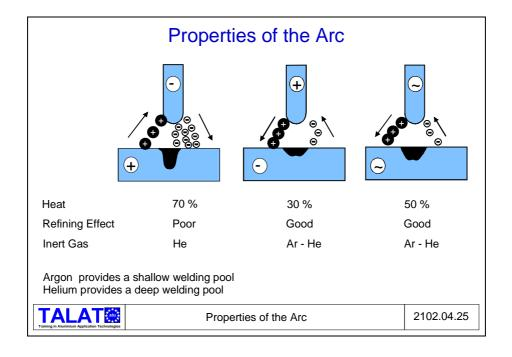
The energy of the welding arc also affects the form of the weld pool. Helium gives deeper penetration, while argon results in more shallow penetration but a broader weld pool. The disadvantage is that helium is very expensive so it is only used in special cases. MIG welding is often performed using a combination of argon and helium. There are manuals available that list the parameters that apply to welding aluminium. Important welding parameters are included in Figure 2102.04.26:
