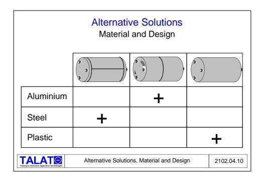
**Steel:** Compressed air tanks are usually fabricated of unalloyed steel. The material's excellent weldability favours welding over deep drawing. This means that alternative A is preferable, although alternative B is also a possibility.
