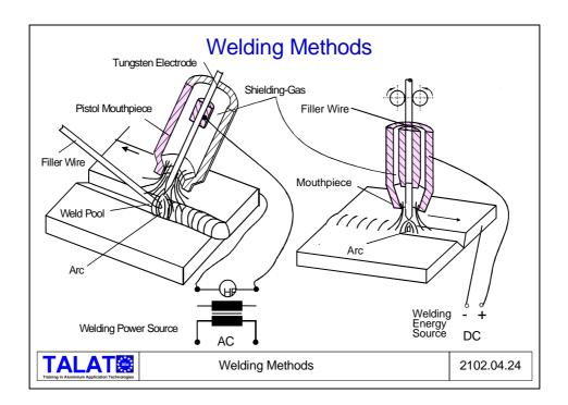
TIG welding uses a permanent electrode made of tungsten. AC current is usually used to prevent overheating. The method works well with thin materials. An added advantage is that it can be used with or without filler material. However, the AC current results in less welding strength than MIG welding.
