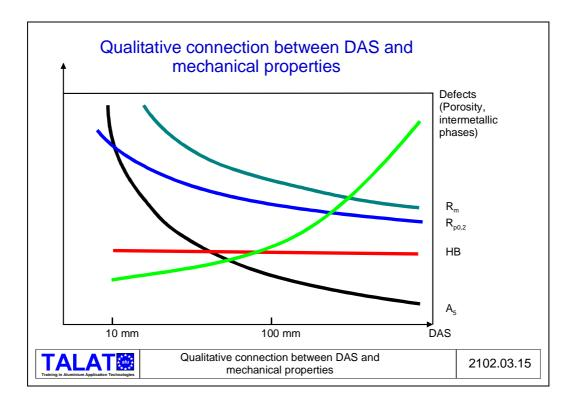
However, the mechanical properties still don't turn out as well as expected. During pressure die-casting, the mould is filled at such high velocity that the turbulent flow causes the metal to trap gas. With gravity die-casting, on the other hand, the mould is filled with a laminar flow, preventing that particular problem. In other words, gravity die-casting actually results in the best mechanical properties.
