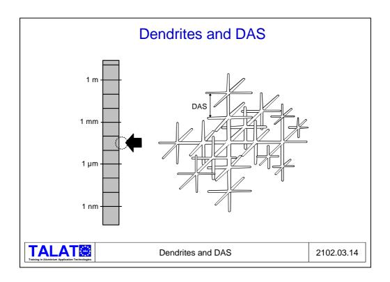
It is therefore essential to perform the casting operation in such a way as to minimise the distance between the dendrites. The speed of cooling (quenching) after casting is the primary factor affecting the dendrite arm spacing. Rapid quenching results in small distances, a fact which favours thin sections and the use of metal moulds. It would therefore appear that pressure die-casting would have a positive effect on the mechanical properties of a cast product (Figure 2102.03.15).
