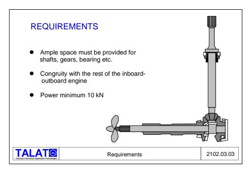
**Ample space** must be provided for shafts, gears, bearings, etc. The product has to be adapted to the dimensions and tolerances that apply.
