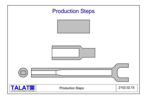
Once the sketches are approved, model tools are made, any adjustments are undertaken and tests are conducted. Then the real tools can be engineered and produced. The next step is a test run. The metallurgical characteristics of the product are examined to discover any propensity to crack, and to observe the product's flow lines and texture. The product's hardness is measured after heat treatment. Finally, the shaft is machined, and torsion and fatigue tests are conducted.
