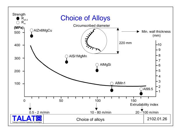
We can see how extrusion speed is influenced by the choice of alloy. The same figure shows how the minimum wall thickness of an extrusion is also contingent on the choice of alloy. The curve indicates the minimum wall thickness. For instance, Al 99.5 has a minimum wall thickness of 2 mm, compared with 3.2 mm for AlSi1MgMn.
