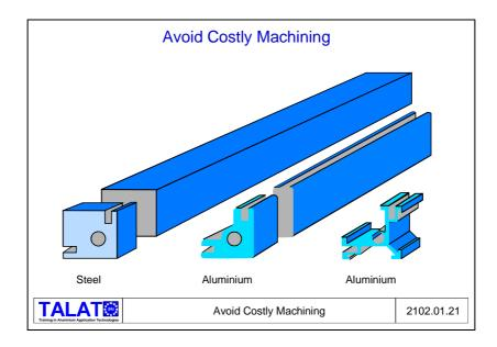
Figure 2102.01.21 gives an example of one specific component which, when made of steel, is produced from steel bar which has to undergo several processing operations. When made of aluminium, it is directly extruded as an integral part of our final cross-section, then finished by simple processing.
