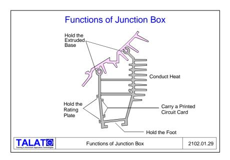
Initially, we planned to weld the junction box to the rest of the light fixture, but eventually we wondered whether there wasn't a better method of assembly. The extrusion expert proposed further improvements. Why couldn't the junction box, which was also to incorporate several functions, be made from an extrusion? **Figure 2102.01.30** gives an idea of the final solution. Ultimately, the junction box was made of an extrusion designed to be slid into place on the extruded casing.
