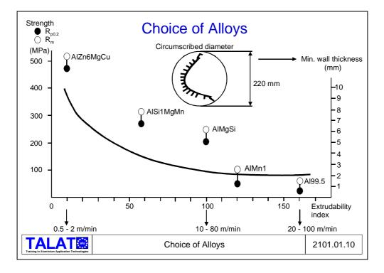
Al99.5 (AA1050) and AlMn1 (AA3103) are not heat treatable. ince extrusion is a hot forming process, these alloys will have very low strength. ubsequent cold drawing of tubes or wire will let us achieve strength attributes comparable to those achieved by cold rolling. These alloys are readily extrudable and can be manufactured as thin-walled sections. However, heat treatable alloys are usually used for extrusions. The diagram
