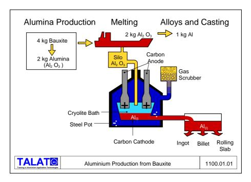
In about 1918, the Norwegian scientist C. W. Søderberg invented a continuous electrode, the "Søderberg cell", which is still in use today. Most modern electrolytic reduction plants now use pre-baked electrodes for environmental reasons.
