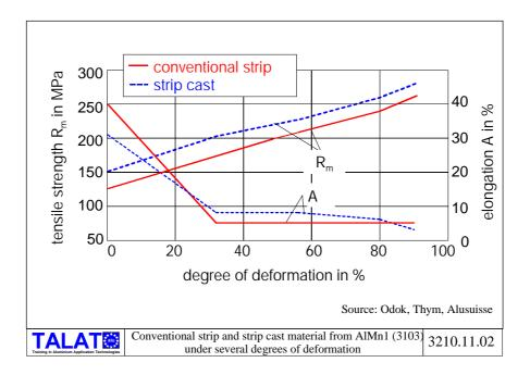
If the alloy content is at about 2% (AlFe2, AlMn1Fe1, see **Figure 3210.11.03**) the ductility can raise with increasing degree of deformation. The reason for this phenomenon is to be seen in the primary precipitations, that build a dense net in the ascast condition. Above 40% degree of deformation this net is broken and the deformation
