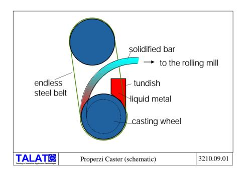
Properzi rod is usually delivered at 12 mm diameter to be drawn by dry drawing machines to a final diameter of 0.3 mm to 4.0 mm depending on the application.
