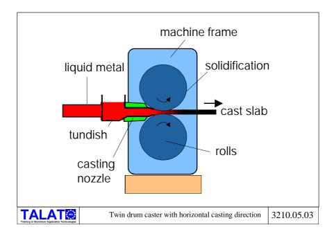
The cast strip emerges horizontally from the caster and is directly wound into coils while hot (**Figure 3210.05.04**). The coil size is adapted to the following cold rolling mill.
