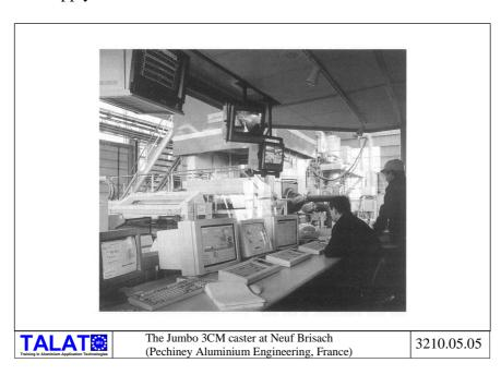
The new developed Jumbo 3CM casting line features a tilting melting/holding furnace, a molten metal feed system including a motorised support table, a tundish and a previously set-up nozzle kit and an automatic level control system in the tundish and nozzle. For some alloys, the last parameter plays an important role because of its influence on the heat exchange between the molten metal and the rolls, which effects on the structure of the skin of the product.
