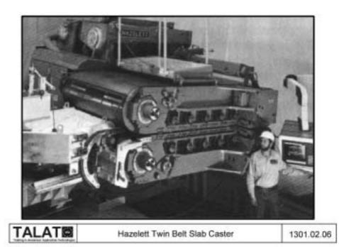
The process is shown schematically in **Figure 3210.04.03**. **Figure 1301.02.06** shows the casting machine. The principle of operation is to pour the molten metal into the space between the belts via a casting nozzle, with the same width as the strip to be cast. In this space between the belts the metal solidifies and is drawn out of the machine by a pinch roll. The casting rate is 5 m/min to 9 m/min.
