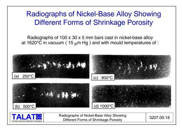
In contrast, as shown in **Figure 3207.00.18**, layer porosity can be seen quite clearly in X-rays, as long as the radiation is oriented along the plane of the porosity. This is because, of course, the radiograph effectively integrates the porosity over the depth of the section.
