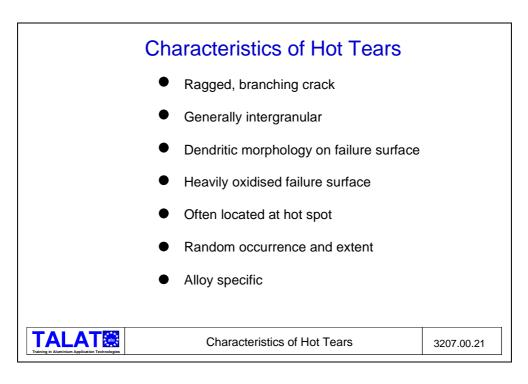
I would now like to turn to hot tears which are one of the most serious defects that can occur in castings. These have a number of characteristics, as shown here (see also **Figure 3207.00.21**):
