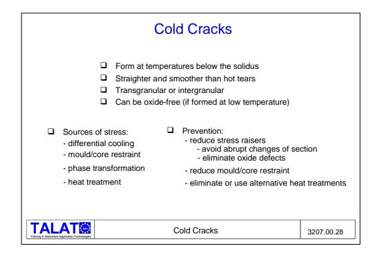
The final type of defect that we will consider are **cold cracks** (**Figure 3207.00.28**). By definition, these form at some temperature below the solidus and often considerably higher than room temperature.
