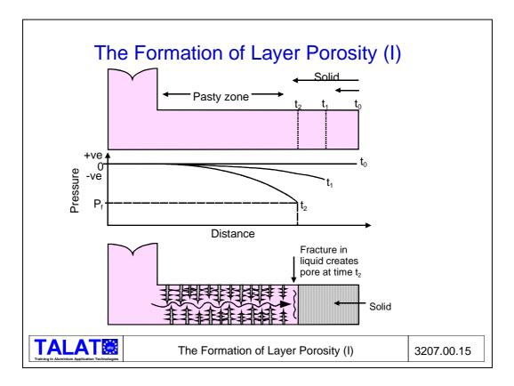
The hydrostatic tension in the liquid in the pasty zone continues to increase until, at time  $t_2$ , a critical fracture pressure  $P_f$  is reached at which a pore will nucleate. This could be an isolated micropore if the shrinkage conditions are not too severe. The generation of small regions of microshrinkage porosity in long freezing range alloys is quite common.
