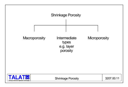
The second type of defect that we need now to consider is **shrinkage** porosity, which is conventionally sub-divided into macroporosity and microporosity (see **Figure 3207.00.11**). In reality, there is no fundamental difference between these two forms of porosity - one gradually changes into the other as a function of the freezing range of the alloy. As we will see, it is also possible to identify intermediate types of shrinkage porosity, notably layer porosity in long freezing range alloys.
