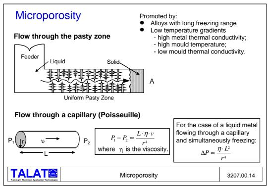
In such cases, towards the end of solidification, there will be a 'pasty' or 'mushy' zone consisting of a forest of dendrites enclosed in the remaining liquid. This shows a simple bar-shaped casting with a feeder at one end. We shall assume that the temperature profile is such that:
