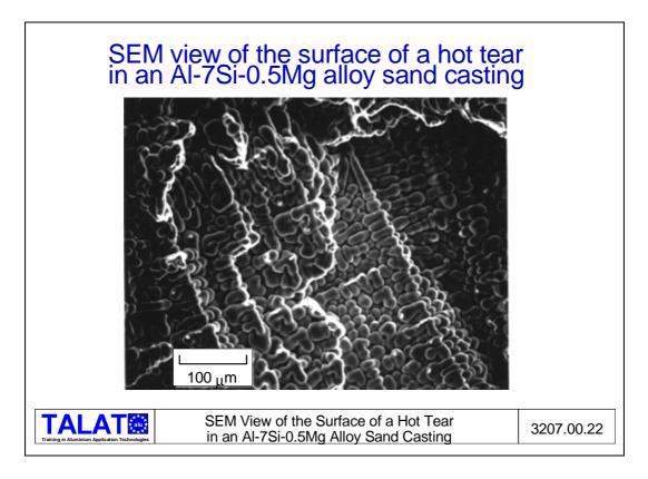
**Figure 3207.00.22** shows the surface of a hot tear in an Al-7Si-0.5Mg sand casting as viewed by a scanning electron microscope. The dendritic morphology is clearly revealed. Hot tears occur in the late stages of the pasty condition of freezing, when only a per cent or so of residual liquid remains between grains.
