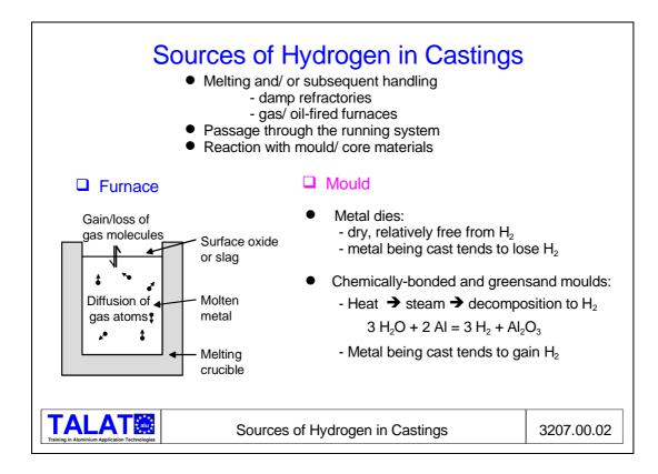
The first type of gas defect that we shall consider is that caused by precipitation of gas from solution in the liquid metal but we will initially need to understand how the gas gets into the metal in the first place (see **Figure 3207.00.02**). In the case of aluminium, we are particularly concerned about hydrogen, which can come from several sources:
