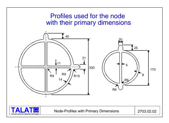
The extrusion for the cord of the node uses an inside wall to take up the transverse load. Together with a part of the tube itself, an effective I-beam is constructed (**Figure 2703.02.03**). This avoids ovalization of the cord and therefore reduces the stress level considerably. To be able to use the profile in a real three dimensional structure, a
