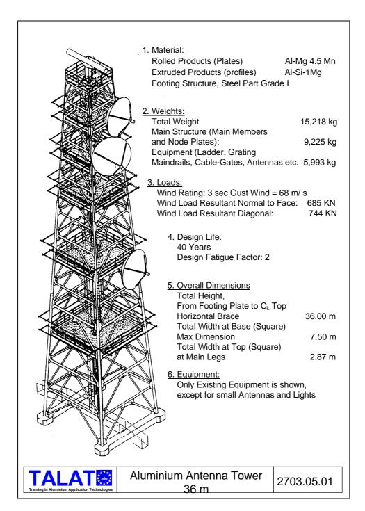
As a consequence of the design work on the antenna tower, the nodes were optimized with respect to fabrication, low node complexity, splicing of members, transition between members of unequal size, transition to steel foundation, supports for secondary structures and equipment, access for inspection and finally weight and cost.
