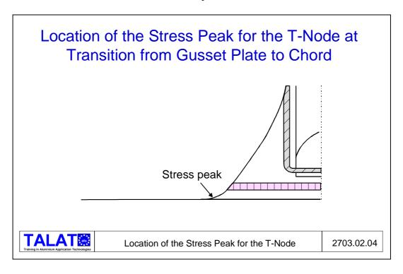
Also the profile for the bracing has integrated a small part of the gusset plate in the extrusion (see **Figure 2703.02.04**). This again removes the weld from the stress peak caused by the start of the gusset plate and is well adapted for manufacture and inspection. The profile has a thin wall inside which prevents ovalization, and corresponding high stress levels in the bracing. Without this inside wall, excessive ovalization of the bracing was seen when optimizing the node.
