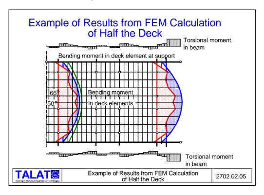
The maximum span for the longitudinal girders is approximately 15,0 m and for the extrusions the span is about 5,0 m.
