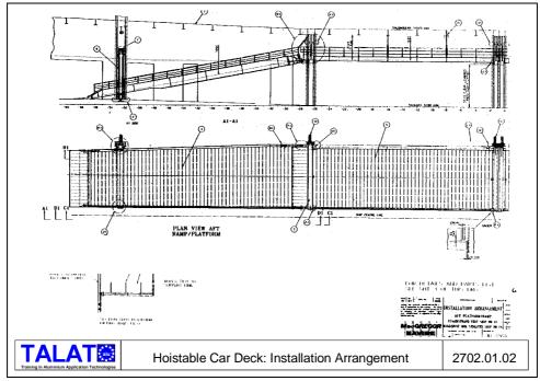
The ramp sections are designed to be raised when loaded with cars. The deck sections
