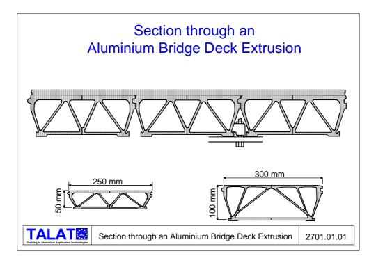
When subjected to concentrated loads, which is most often the case for bridge decks, the resistance of the deck is due to a combination of the bending and torsional stiffness of the extrusions. In this way the load distribution will be considerable and concentrated loads will be carried by at least seven extrusions at the same time.
