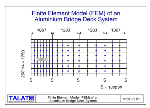
Here, the applied load is represented by a pair of truck tyres. The load was placed in the most unfavourable position to cause the largest possible deformation in the structure, as shown in **Figure 2701.02.02**. The deformation reached a maximum of 6.5 mm at the
