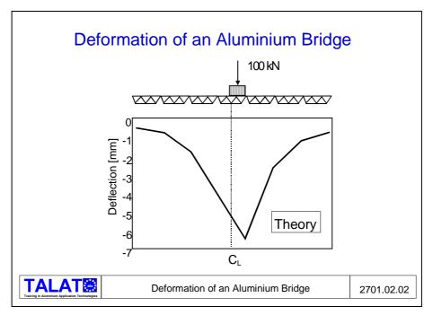
A full-scale model was tested to confirm the results of the theoretical investigations. These tests included static loading as described above and dynamic loading in accordance with the requirements set by the Swedish National Road Authority.
