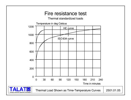
To determine the fire resistance of a construction or partition, standardized fire tests can be performed. In a fire test the specimens are put on, at or in a furnace which is capable of subjecting the test specimens to the standardized thermal load. A test procedure (**Figure 2501.01.06**) is described in ISO 834 [5].
