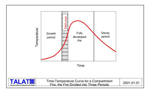
As shown in **Figure 2501.01.01** a fire in a room goes through 3 phases [1]:
