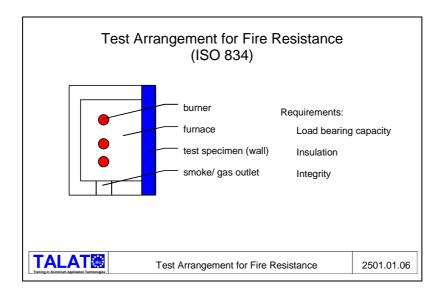
The test specimens shall be heated in the prescribed manner until failure occurs under any one of the relevant test requirements:
