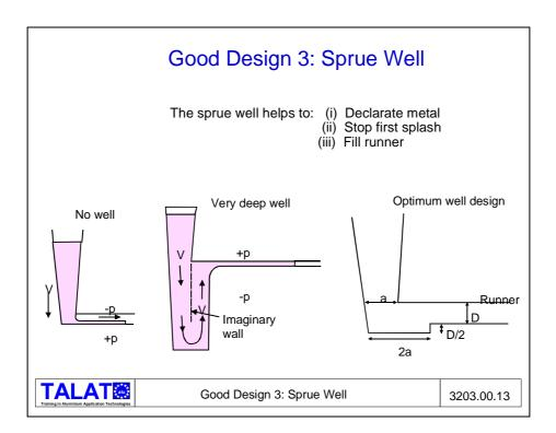
If there is no well, the falling metal stream hits the bottom surface of the runner bar at a velocity V and spreads along the bottom surface of the runner (see **Figure 3203.00.13**). In doing so, it creates a pressure, + p, which is balanced by a negative pressure, - p, on the top surface of the runner bar. This tends to draw in air through the permeable sand mould, leading to oxidation of the metal.
