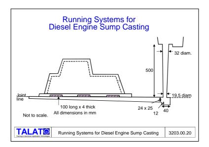
**Figure 3203.00.20** shows the calculated dimensions of the runner system. It has been assumed that square sections are used for the sprue and runner, although other cross-sectional shapes could be used, so long as the areas are correct. The remaining important feature to be designed is the well base which is based on the optimum dimensions which have already been defined in **Figure 3203.00.13**.
