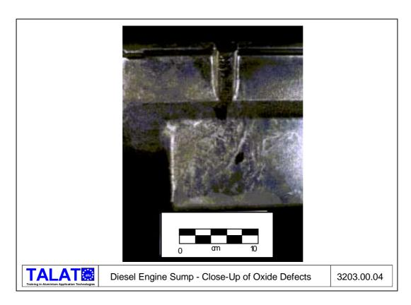
The fact that these oxide film defects often cause castings to fail leak tests clearly implies that the defects are continuous from one side of the casting to the other. Castings are normally tested by pressurising them with air whilst they are submerged under water so that the defects are revealed by a stream of bubbles. The operator then attempts to seal the porosity by peening over the surface, leaving these tell-tale marks on the casting surface (**Figure 3203.00.05**).
