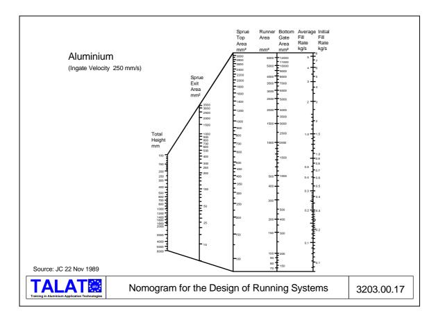
**Figure 3203.00.17** is a nomogram for the design of running systems for aluminium castings and will ensure that the maximum ingate velocity does not exceed 250 mm s<sup>-1</sup>. This is half the critical velocity and will therefore provide a certain safety margin.
