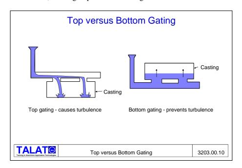
**Figure 3203.00.10** shows another common mistake, in which the metal is introduced into the top of the casting cavity, i.e. by top gating. The critical velocity is readily exceeded and the resulting turbulence and splashing cause oxidation of the molten metal. The preferred technique is to use bottom gating, i.e. to introduce the metal uphill into the casting although, as we will see, it is still important to limit the velocity with which the metal enters the mould.
