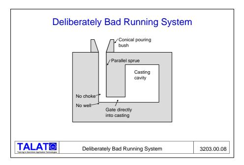
This a section through a mould and shows four deliberate mistakes, namely a conical pouring bush, a parallel sprue, no choke and no runner bar, so that the metal enters directly into the casting. We will now consider the effect of these bad design features.
