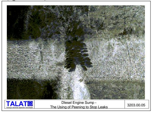
The lesson to be learnt from this is that castings in metals such as aluminium should not be top-poured. The remainder of this lecture is concerned with how to fill a casting without creating this mess of entangled oxide films.
