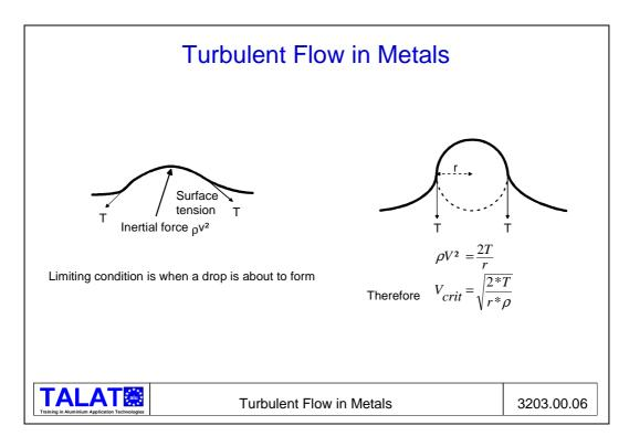
The limiting condition can be seen to be when the inertial force is balanced by the surface tension force, i.e. when
