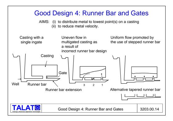
The well should be the lowest point of the casting and filling system and the metal should always progress uphill thereafter (**Figure 3203.00.14**). In doing so, it firstly passes through the runner bar which distributes it through gates to the lowest point or points on the casting. Careful thought has to be given to how the metal will flow through the runner and casting, bearing in mind the need to keep the speed low in order to avoid surface turbulence.
