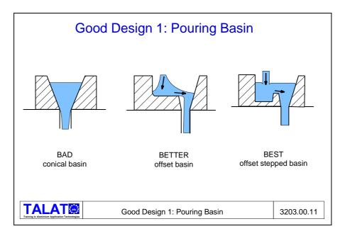
The best design is to introduce a step into the basin to give an *offset stepped basin*. The step acts to stop the rapid motion of the metal over the top of the sprue and helps to ensure that the latter is completely filled.
