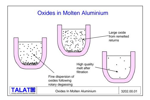
In fact, it is necessary to develop of view of the liquid as a slurry of sundry solid debris in suspension. It is only the size and quantity of solid debris which is changed from melt to melt and from one melting practice to another. In particular, we will see how the large oxide films which may be present from remelted returns can be substantially reduced by rotary degassing and filtration.
