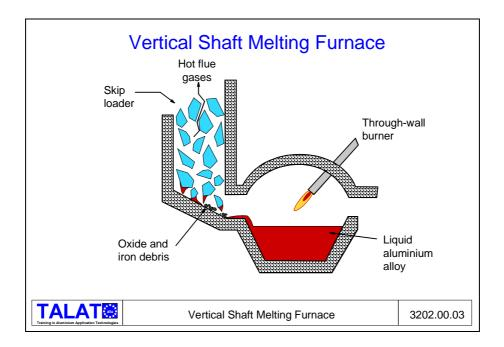
Having started with a reasonable quality of liquid metal, it is necessary to try to keep it in good condition. However, it is again with regret that it has to be reported that most aluminium foundries do not achieve this. (It is achieved in casting houses designed for the continuous casting of wrought quality aluminium alloy, especially that to be used for such discriminating applications as foil or can stock.)
