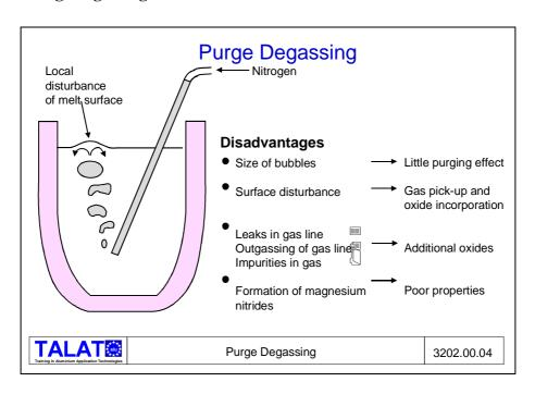
One such treatment is degassing (see **Figure 3202.00.04**). This is often carried out badly, using an open-ended lance to introduce a purge gas into the melt.
