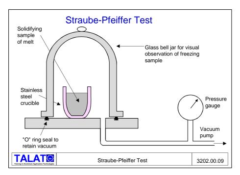
The reason for carrying out the test under reduced pressure is simply for the convenience of the magnification of the volume of gas by a factor of ten (or more if carried out at lower pressure; a factor of 30 is rarely exceeded). The pores are much more easily seen as they emerge at the surface, and are easily visible when the sample is cut up for subsequent examination.
