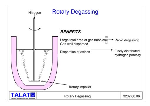
Because rotary degassing is a relatively new technique, little investigative work has been carried out on it so far. There seems to be evidence that the system causes large oxide films to float out, and maintains them at the surface so that they can be skimmed clear after degassing.
