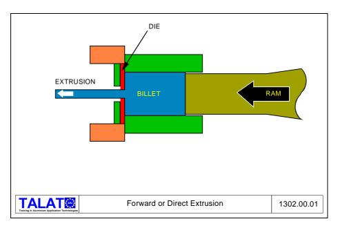
The versatility of the process in terms of both alloys available and shapes possible makes it one of the most valued assets in helping the aluminium producer supply users with solutions to their design requirements.
