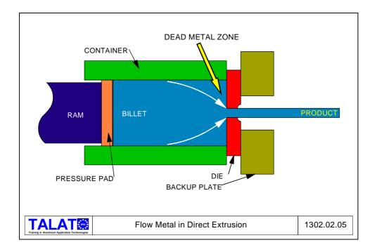
In forward or direct extrusion the ram pressure not only has to deform the metal but also overcome the friction between the billet and the container. With the indirect process the billet and container do not move relative to each other and so all of the available press load is used for deformation. In consequence of these differences indirect extrusion has the following advantages:
