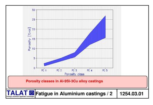
The consequence is clear: porosity has to be minimised; this is the goal of innovative foundry processes for Al alloys. If a comparison is carried out among semisolid casting and more conventional processes, the fatigue behaviour of the semisolid cast alloys is significantly better, due to the strong reduction of porosity which is assured.
