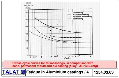
Due to the sensitivity of fatigue properties to defect geometry, the aspects related to size and shape of porosity have to be taken into account, as well as that of the maximum size pore. The failure of the alloy under fatigue depends on these factors: two materials belonging to the same porosity class (i.e. having the same average amount of porosity) but having small sized and round pores the first one and irregular big size porosities the second one are completely different.
