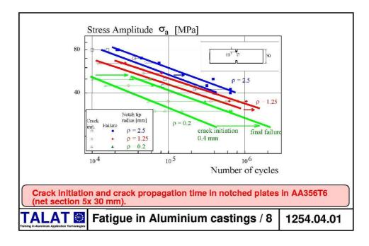
Since crack growth rates of sufficiently long cracks (in this case longer than 0.4 mm) are sufficiently well described by the *Paris law* within linear elastic fracture mechanics, then crack propagation cycles can be estimated by means of the procedures described in TALAT lectures 2400.
