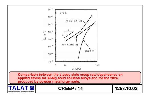
1253.11 Creep-resistant Al-base Materials: High-strength Powder Metallurgy- Dispersion-strengthened Aluminium Alloys
