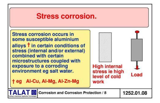
There are three conditions which are essential to cause stress corrosion cracking:
