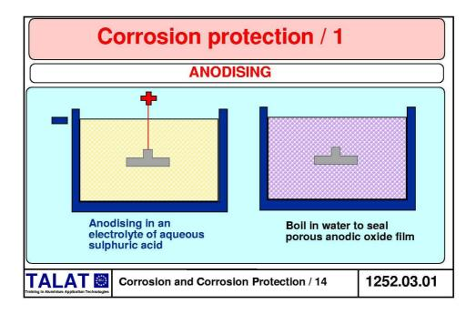
In a number of electrolytes, e.g. dilute sulphuric, chromic, oxalic and phosphoric acids, the reaction products on aluminium anodes are sparingly soluble and strongly adherent.
