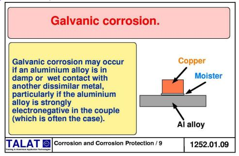
If an aluminium alloy is in contact with another metal in the presence of moisture then electrolytic corrosion may occur.
