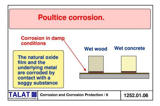
This is caused by contact with a wet soggy substance. The substance may have chemicals in it which may accelerate the attack. Usually this is a customer problem due to either bad design or maintenance.
