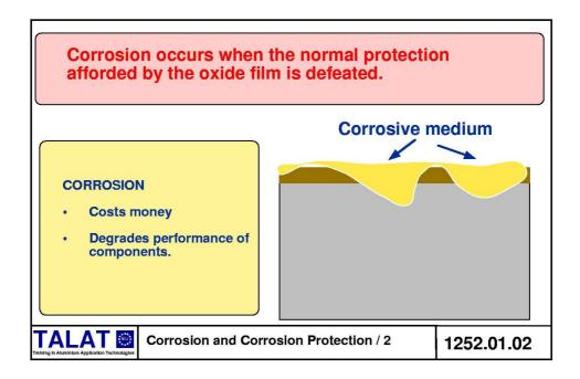
Consequently, it is important to understand the circumstances under which corrosion may occur and also how such corrosion may be prevented.
