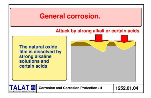
The natural oxide film on aluminium dissolves in strong alkaline and certain strong acid solutions. For example, severe attack occurs in concentrated sodium hydroxide (caustic soda) solution and in dilute nitric acid - for a comprehensive list, see reference [3].
