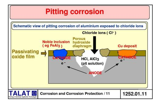
Pitting is localised galvanic corrosion and is caused by the occurrence in the base alloy of inclusions, or regions of different composition, with an electrochemical potential different from that of the matrix.
