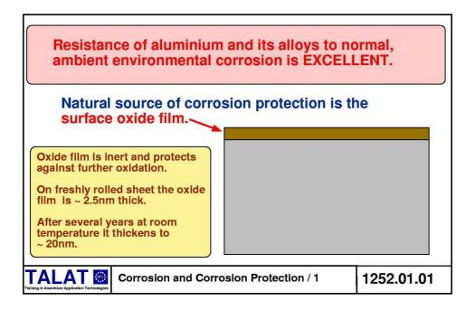
Although aluminium is reactive, the oxide film that forms on it is inert and protects it from further oxidation. The oxide film is about 2.5nm thick on fresh rolled sheet and it builds up over several years to some 10-20nm  $(1nm = 10^{-9} \text{ m})$  in thickness.
