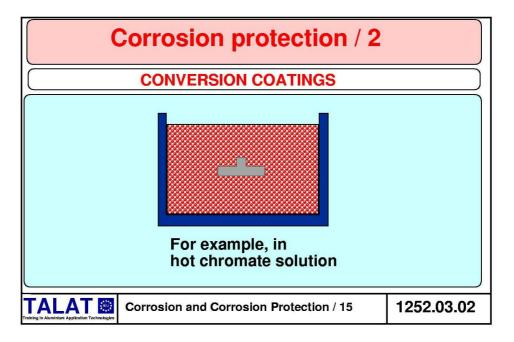
In this case fluorides are added to the chromic acid to remove the initial  $Al_2O_3$  and allow the local cell action to proceed. With phosphoric acid this anodic product is an aluminium phosphate.
