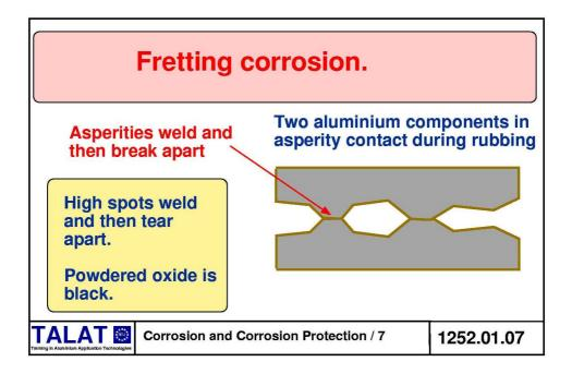
Fretting corrosion manifests itself as black spots on the metal surface underneath which can be deep pits.
