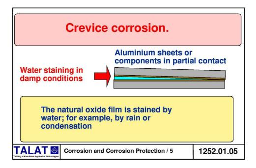
This is often known as water staining. There are two main conditions which will induce crevice corrosion:
