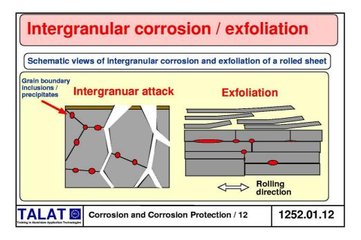
Normally an aluminium solid solution is reasonably resistant to general corrosion, protected as it is by its oxide film.
