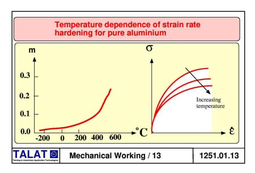
Note that aluminium alloys that are formable by superplastic deformation have strain rate sensitivities > 0.5. A stable, fine scale microstructure is required for superplastic deformation, by which ductilities of several hundreds of percent are possible. This requires special alloy compositions, containing Zirconium which provides particles which pin grain boundaries, Figure 1251.01.14.
