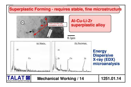
In heat treatable aluminium alloys, the <u>effective hardening precipitates</u> are very small and it is necessary to use TEM to observe these directly, see TALAT <u>lecture 1204</u> on precipitation hardening. Also the small sub-micron *dispersoid particles* present in some alloys are observable only by TEM.
