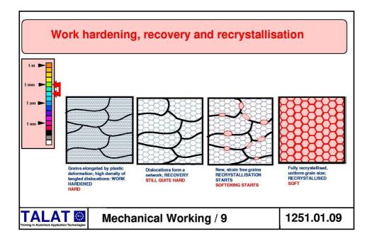
The driving force for recrystallisation is the *stored energy* caused by the presence of dislocations, **Figure 1251.01.10**.
