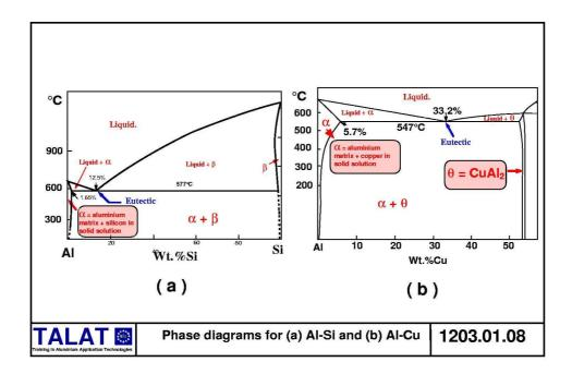
The Al-Cu system is important as a classical precipitation hardening system for alloys of up to  $\sim$  4wt% Cu, and we will look in much more detail at this system in the next **lecture 1204**. It is to be noted that the equilibrium eutectic phases are  $\alpha$  and  $\theta$ , where  $\theta$  is the intermetallic phase CuAl<sub>2</sub>.
