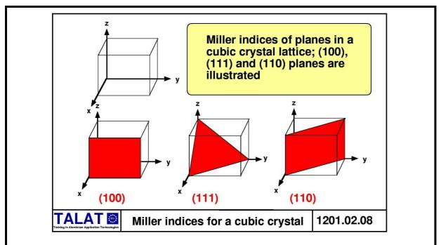
Directions in the cubic crystal are defined in 'square brackets' as the normals to the planes; for example, the direction along the x- axis is [100]. A family of equivalent 'cube' directions is denoted as <100>.
