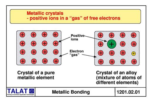
The free electrons in the "electron gas" of a metal are relatively free to move. Under the influence of a voltage potential, an electron current flows. Hence, metals are good conductors of electricity.
