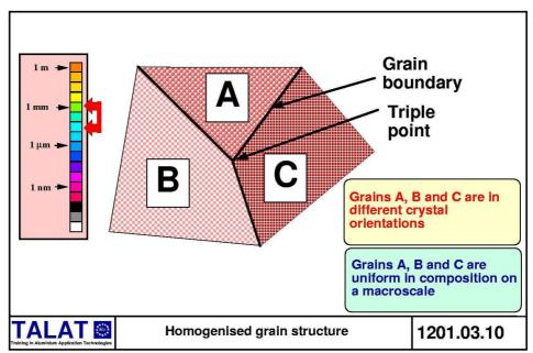
The boundaries between grains are in a state of local, high disorder and are of higher energy relative to the regular lattice of grain interiors. Thermodynamic principles say that systems always tend to minimise their total energy; consequently, a sustained annealing treatment leads to growth of grains to lower the total grain boundary area. This same principle is the main driver that determines how a material responds to deformation (working) and further heat treatments.
