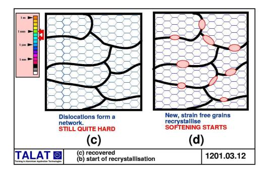
*Recrystallisation.* If the temperature of the slab is raised further, new strain free crystals are nucleated; recrystallisation has commenced, **Figure 1201.03.12**. and the material starts to soften. This process continues until the whole of the material has recrystallised and softened, **Figure 1201.03.13**.
