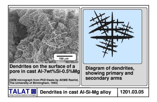
Let us start by considering the freezing (solidification) of an aluminium alloy. As the liquid cools to, and then below, the freezing point, small crystals of solid start to grow within the liquid. The solid crystal grows at different rates in different lattice directions - in aluminium, as for all fcc metals, the preferred growth directions are the cube <100> directions, and the
