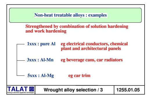
Pure aluminium (1xxx series) finds applications in electrical conductors, certain plant for chemical engineering and for architectural panels. Tensile properties are low in the annealed condition ( $\sim 50 MPa$ ) and can be doubled by cold work.
