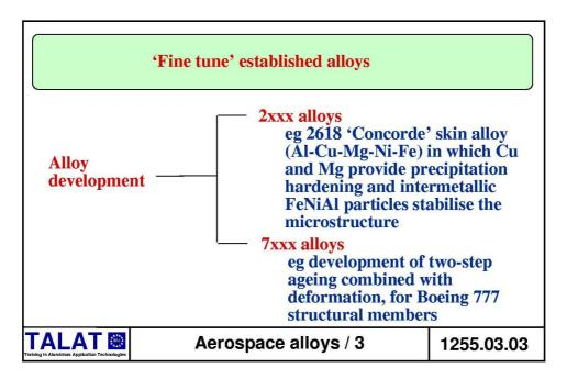
2xxx series alloys continue to be used as aircraft structural materials, for example as fuselage skins. Enhanced fracture toughness has been achieved by improvements in alloy cleanness, for example, lower levels of iron and silicon. Alloy 2618 (Al-2.2Cu-1.5Mg-1Ni-1Fe) is used as the fuselage skin of Concorde, with the Cu and Mg providing precipitation hardening and FeNiAl<sub>9</sub> dispersoid particles stabilising the microstructure [1].
