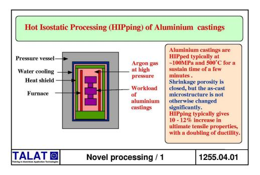
Hence, HIPping may be seen as a method of counteracting the natural interdendritic porosity that occurs during solidification of an aluminium casting.
