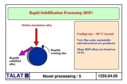
Al-Fe with Fe contents around 8% are commonly used as the base for RSP aluminium alloys. Fe has virtually no equilibrium solubility in Al, see **TALAT lecture 1203** and **Figure 1203.01.09**. However, by very rapid solidification the Fe may be forced into high metastable solid solution, which then precipitates fine-scale metastable phases which confer useful mechanical properties on the alloy - particularly higher strength at elevated temperatures of around 300°C to 400°C [1].
